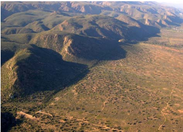
Figure 1. View ENE along the bush-covered trace of the Kango fault separating the pre-Cape and Palaeozoic rocks of the Swartberg Mountains at left, from Mesozoic basin fill and thin Quaternary to Holocene cover sediments, at right. The trench at left foreground was excavated across a locally-developed, elongate, 32m wide graben that truncated the proximal reach of a southward-draining coarse-grained alluvial fan.
